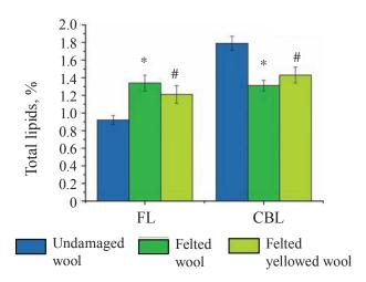
Fig. 2. The total lipids content of undamaged, felted and felted yellowed wool (FL – free lipids, CBL – covalently bound lipids). This and on Fig. 3-4 \* difference between undamaged and felted wool is significant; # difference between undamaged and felted yellowed wool is significant,  $P \le 0.05-0.001$
